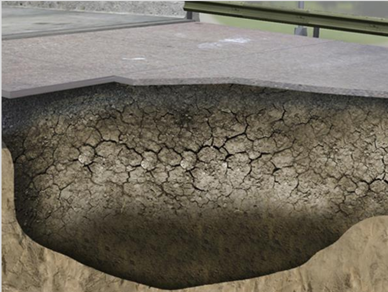
Poor Soil Consolidation
